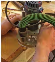
Shoulders first. A shallow rabbet is cut on each side of the shelves to start the making of the tenons.
